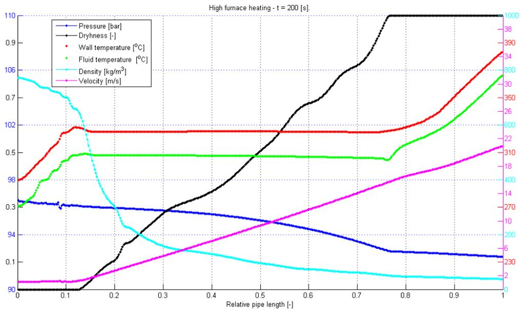
Figure 15: Top firing in SKV3 boiler, after 200 [s].
