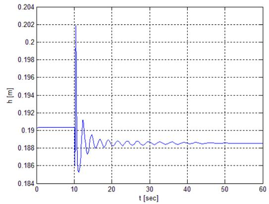
(b) Fluid I: Time evolution of measured depth, 22<sup>nd</sup> cell.
