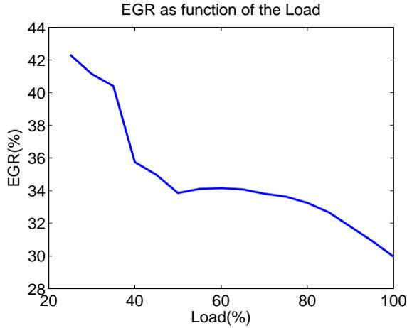
Figure 2: Recirculation percentage as function of the load.
