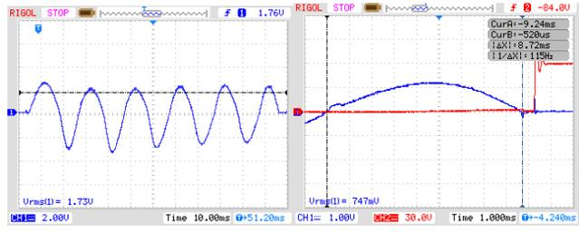
Fig 5. Test 1:TRV Voltage and current in TO CB at the last half cycle Fig 6. Current through TO CB, sampling
