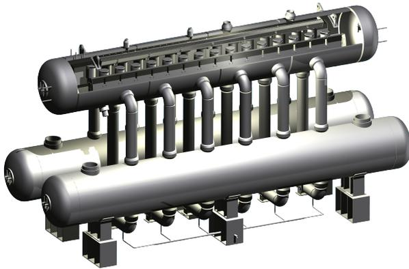
Figure 1: Steam generation system of the CSP plant.[3]
