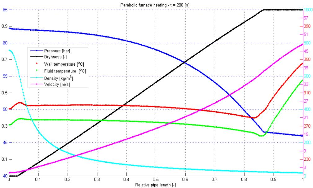
Figure 23: Parabolic heating in SKV3 boiler after 200 [s].
