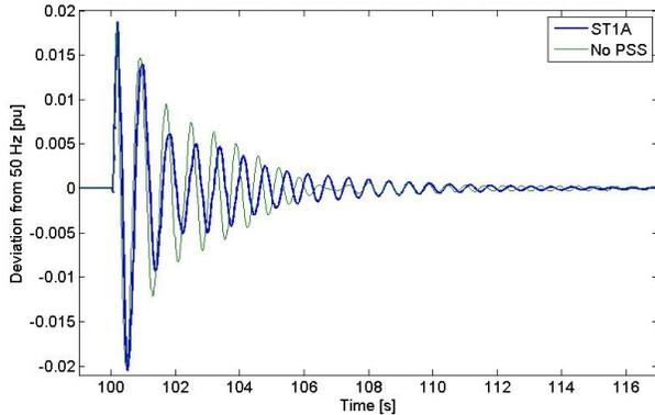
Figure 6: Rotor oscillations at G3 in Dymola
