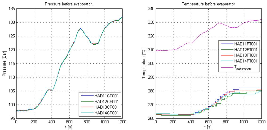
Figure 30: Pressure and temperature after ECO - sample 3.
