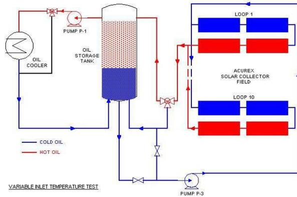
Figure 1: Layout of the Acurex solar collector field.
