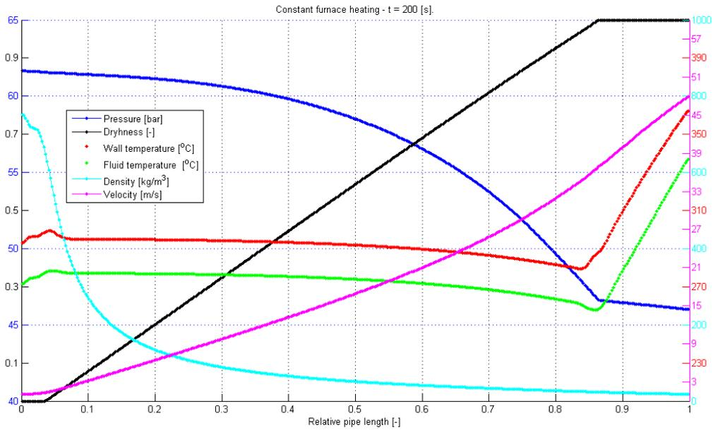
Figure 16: Constant heat flux to boiler, after 200 [s].
