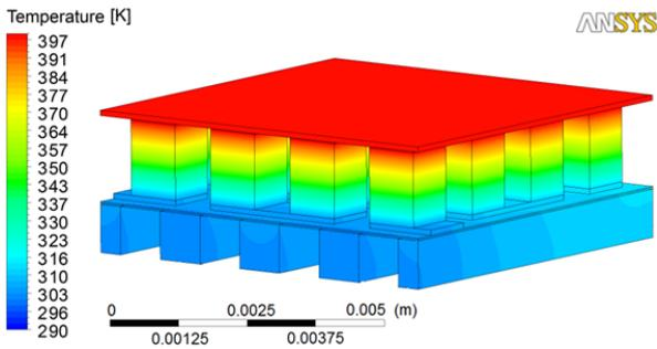
Fig. 3 Temperature distribution in the TEG and fins of heat sink.  $Re = 10$ .
