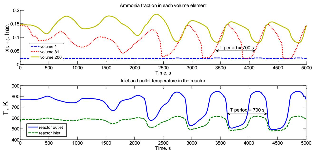
Figure 3: Step response of ammonia fraction and reactor inlet and outlet temperatures when changing temperature of the fresh feed to heat-exchanger from 250 to 200 °C.
