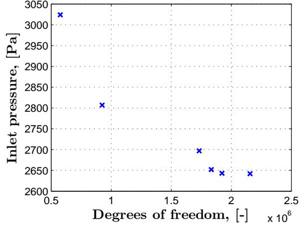
Figure 3: Grid independency study at 298 K
