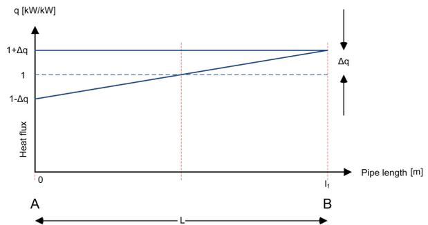
Figure 7: Top firing in boiler with linear heat flux to boiler.
