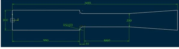
Figure 5: Flume dimension [11].
