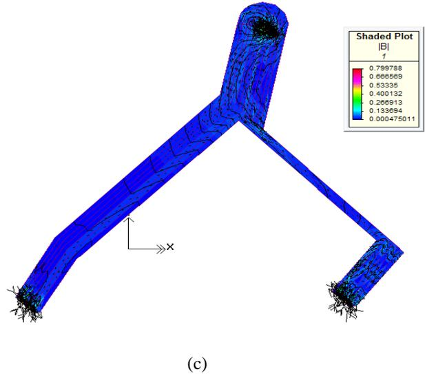
Figure 10. Flux distributions in end area with transposition. (a) Circumferential external flux (b) internal flux (c) external and external flux
