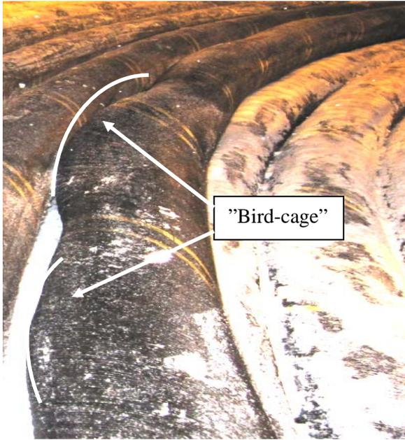
Figure 3: Cable with “bird-cage” [1]
