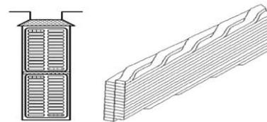
Figure 2. Easy structure of a Roebel bar [5]
