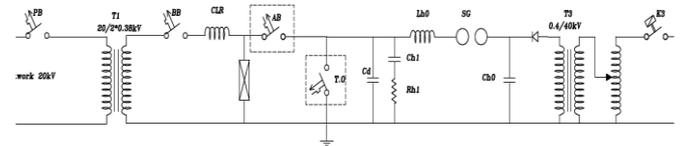
Figure 1. A synthetic test circuit presented by JDEVS.
