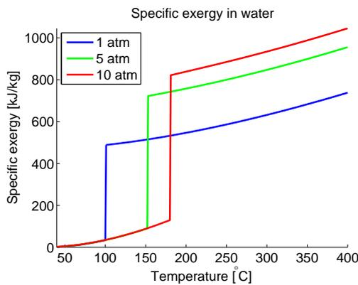
Figure 6: Development of Specific exergy with temperature.
