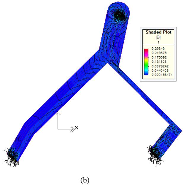
Figure 9. Flux distributions in end area before of transposition. (a) Circumferential external flux (b) internal flux (c) external and external flux
