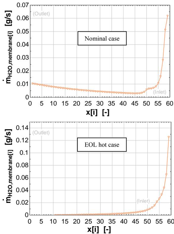
Figure 12: Nafion membrane water transport.
