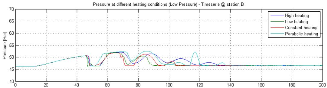
Figure 36: Comparison of the firing profiles on the SKV3 evaporator with respect to fluid pressure.
