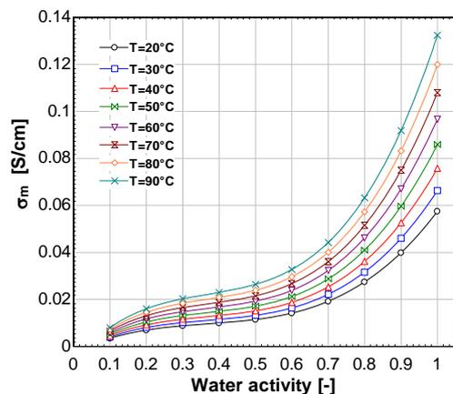
Figure 2: Nafion  $H^+$  conductivity vs. activity & temperature.
