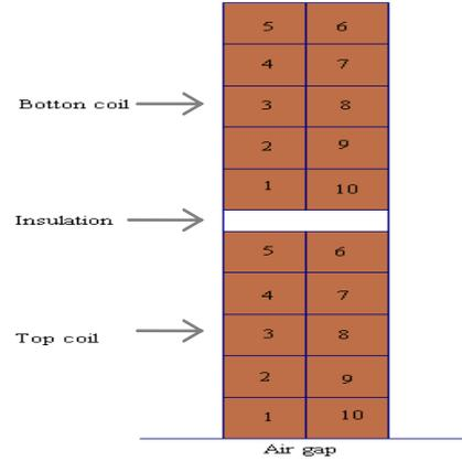
Figure 1. Copper wire order in the simulated model
