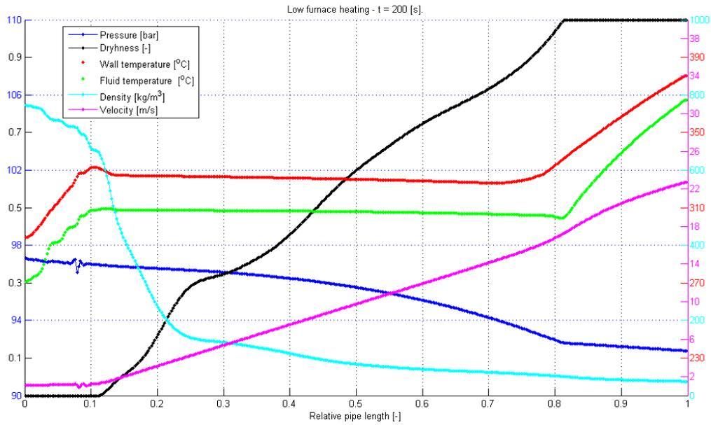
Figure 14: Bottom firing in SKV3 boiler, after 200 [s].
