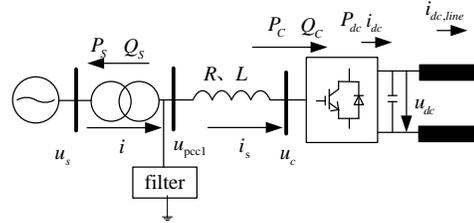
Figure 2: The voltage source converter in DC grid
