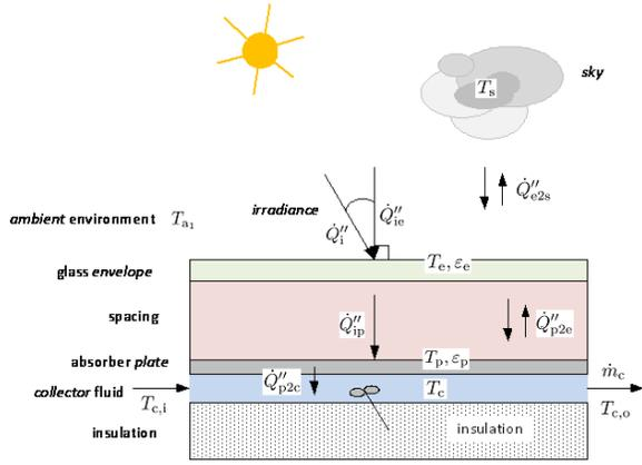
Figure 5: Sketch of collector system with some notation.
