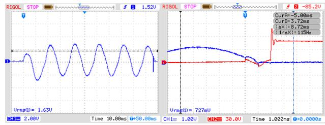
Fig 7. Test 2:TRV Voltage and current in TO CB at the last half cycle Fig 8. Current through TO CB, sampling
