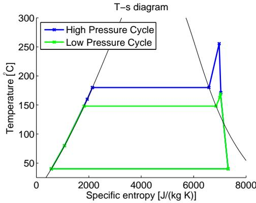
Figure 5: T-s diagram.
