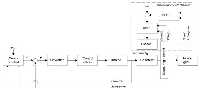
Figure 1: Single generator voltage and frequency control
