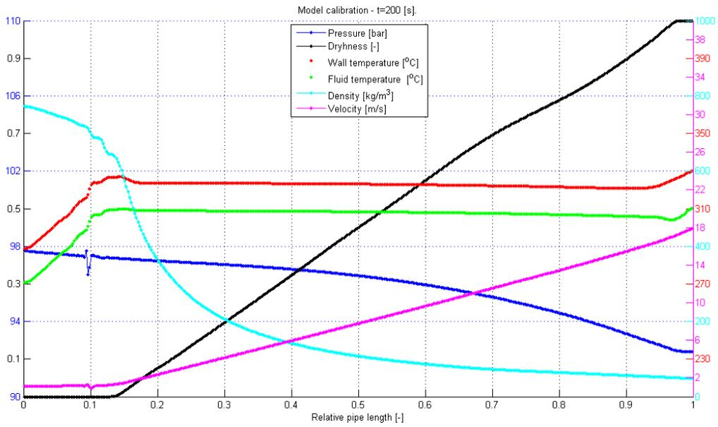
Figure 10: Line series of heat pipe calibration, t=200[s].
