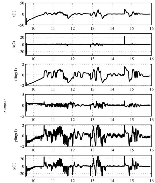
Figure 6: Operation of the LE controller on a cloudy day:  $x = [e, \Delta e]$ ,  $xling = [\tilde{e}, \Delta \tilde{e}]$ ,  $yling = \Delta u$  and  $y = \Delta u$ .
