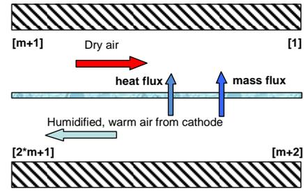
Figure 6: Modeling domain of the humidifier.
