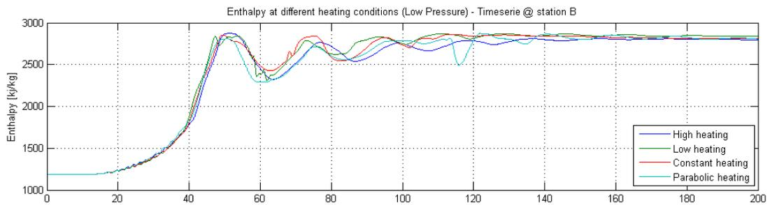
Figure 37: Comparison of the firing profiles on the SKV3 evaporator with respect to fluid enthalpy.
