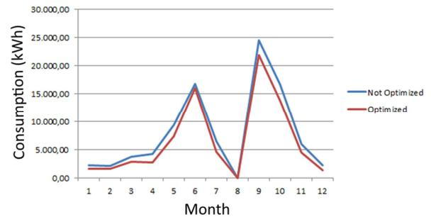
**Figure 13: Cooling consumption extrapolation consumption is given in kWh.**
