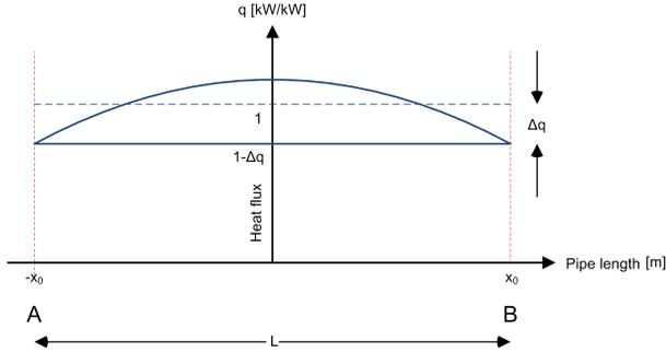
Figure 8: Normal firing in boiler with weak parabolic heat flux to boiler.
