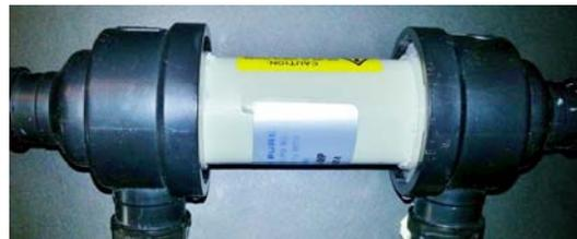
Figure 4: Shell and tube membrane humidifier.
