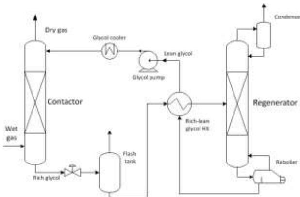
Figure 1: A traditional TEG dehydration process
