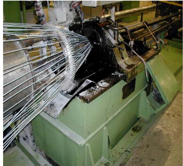
Figure 2: Wires being coated with bitumen
