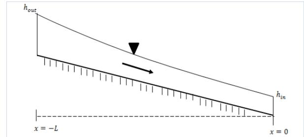
Figure 3: Boundary conditions for computing subcritical flow.
