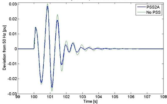
Figure 5: Rotor oscillations at G3 in PSS®E
