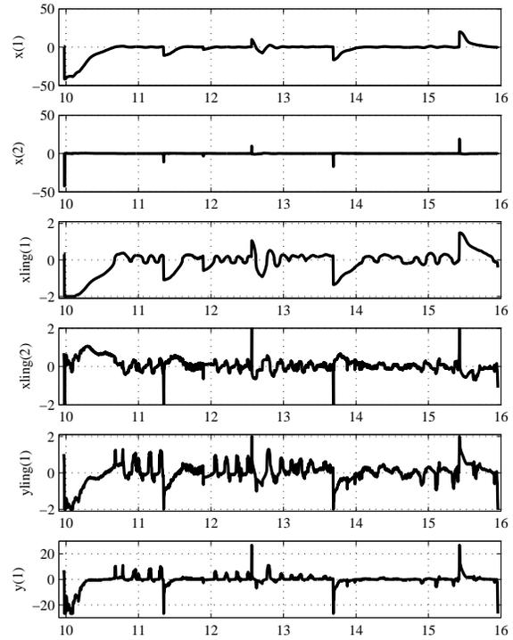
Figure 8: Operation of the LE controller on a clear day, including asymmetry action:  $x = [e, \Delta e]$ ,  $xling = [\tilde{e}, \Delta \tilde{e}]$ ,  $yling = \Delta \tilde{u}$  and  $y = \Delta u$ .
