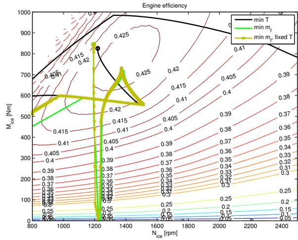
Figure 3: Torque-engine speed trajectories for the three benchmark problems.
