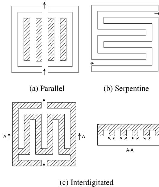
Figure 1: Three archetype channel configurations for square-planar cells
