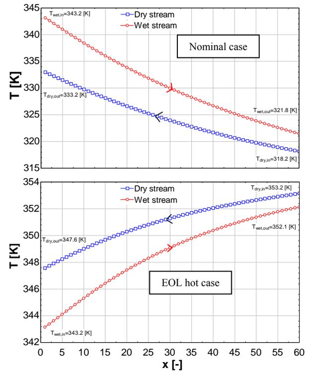
Figure 7: Temperature profiles in humidifier.
