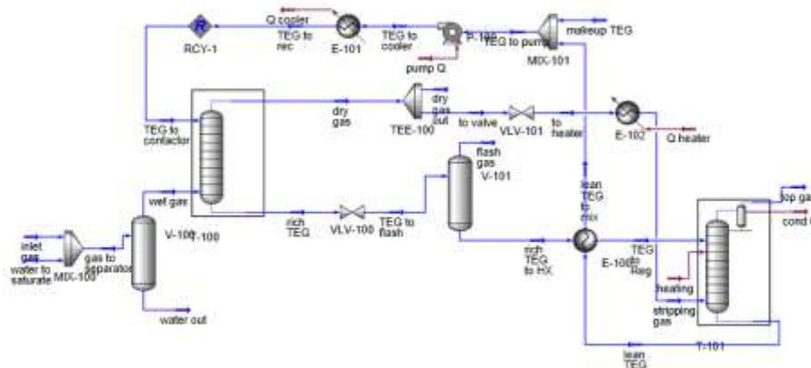
Figure 8: Aspen HYSYS simplified flow-sheet of process with extra stripping column
