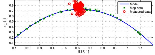
Figure 6: BSR model and its fit to map and measured data
