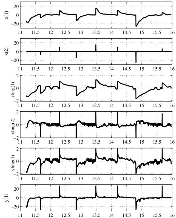
Figure 4: Operation of the LE controller on a fairly clear day:  $x = [e, \Delta e]$ ,  $xling = [\tilde{e}, \tilde{\Delta e}]$ ,  $yling = \tilde{\Delta u}$  and  $y = \Delta u$ .
