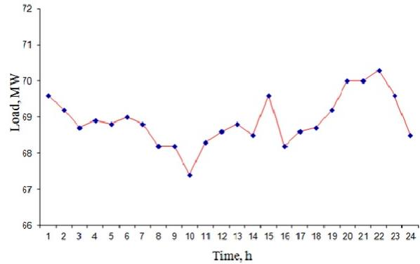
Figure 2: Load curve of the fertilizers plant
