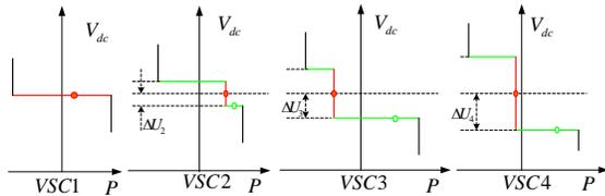
Figure 5: Operation and control characteristics of the DC grid
