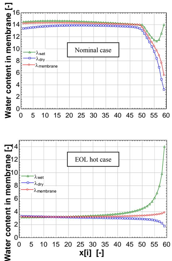
Figure 9: Membrane water contents.
