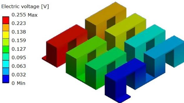
Fig. 4 Generation of the electric voltage in TEG.  $R = 10$ .
