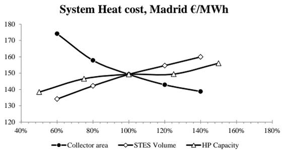
Figure 10: System heat cost depending on collector area, STES volume and HP capacity, Madrid.
